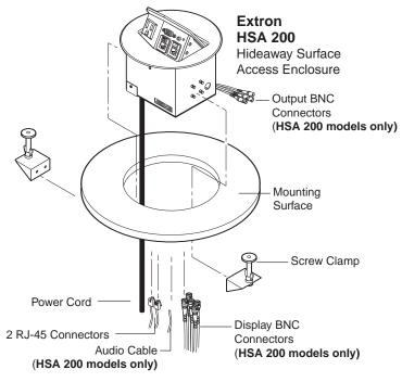
Figure 2-4 — Mounting the HSA 200 or HSA 222 enclosure
